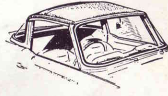
The 'Surrey Top' (a folding canopy of p.v.c.) quickly clips into position for emergency weather protection.
